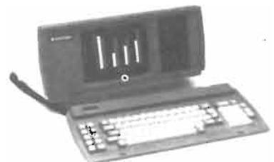
TeleVideo TPC II IBM PC compatible portable computer.
